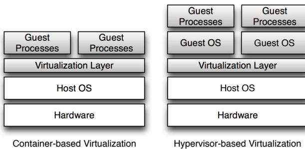
Figure 1. Comparison of container-based and hypervisor-based virtualization.
