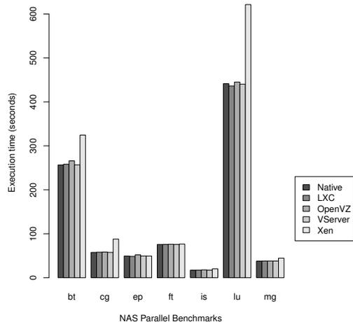
Figure 5. Single node comparison of NPB performance overhead.
